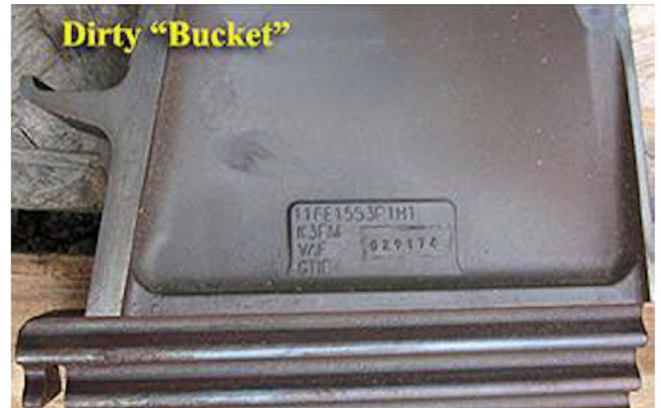
Turbine Bucket before
