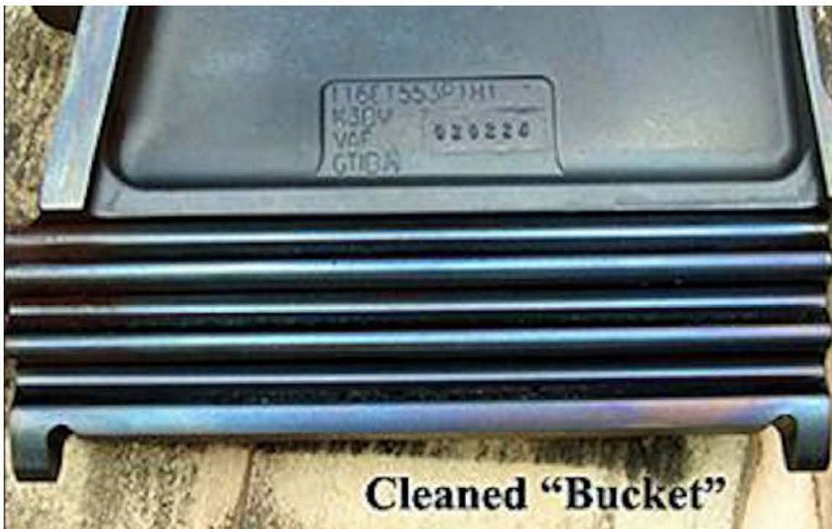
Turbine Bucket after
