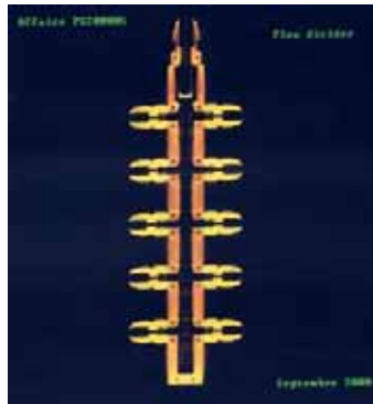
Part internals check by tomography
