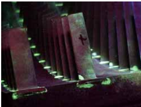
Fluorescent penetrant inspection on heavy duty turbine compressor
