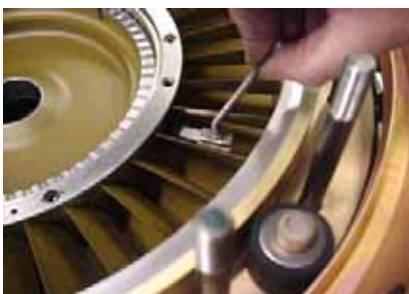
Reassembly of a Centaur compressor
